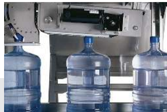
BOTTLED WATER FILL LINES
