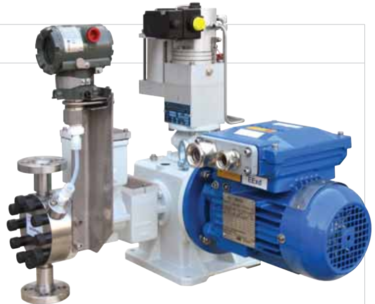
LYHX9 with AISI 316L: pump head being used in Kashagan Field Development (Agip Kazakhstan North Caspian Operating Company), equipped with pneumatic servo with I/P converter and diaphragm rupture detector via pressure transmitter.
