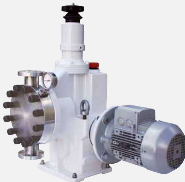
XL pump with single diaphragm and PVDF wetted parts. Automatic adjustment of the flow rate via OBL-designed electrical actuator that being IP66 and thanks to the anticondensation heater, turns out to be suitable for installation in harsh environments such as saline and/or desertic areas with high humidity and wide temperature variation.
