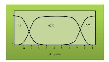
At approx. pH 6, neutralisation starts, and the Hypochloric acid is transformed into Hypochlorite ion - CIO-. At pH 9 and higher almost all Hypochloric acid has turned into Hypochlorite salt. Our Chlorine measurement measures only hypochloric acid.
