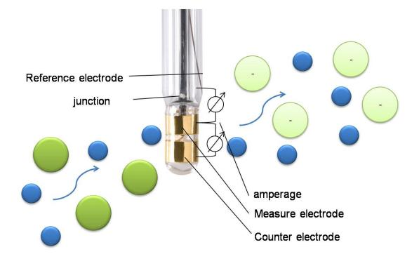
The electrodes of the sensors are made from very high-quality, chemically inert materials such as glass, carbon, and precious metals. These electrodes are in direct contact with the water to be measured. Compared with membrane-covered sensors, this design has several advantages:
