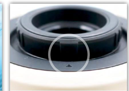
Please make sure that the raised area on the adapter is in line with the triangle\*arrow on the PrimeLab 2.0
