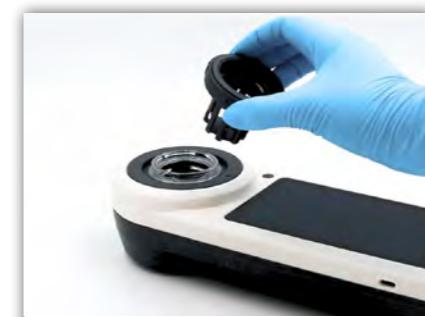
Place your chosen adapter in the transparent protective cup of the smartchamber. Push the adapter down to fix it in place.
