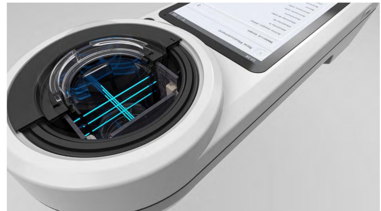
Whilst normal photometers perform tests on one selected wavelength only, the PrimeLab 2.0 receives data from 18 different wavelengths with each measurement, covering the key parts of UV and IR section of the spectrum and the full VIS range.
