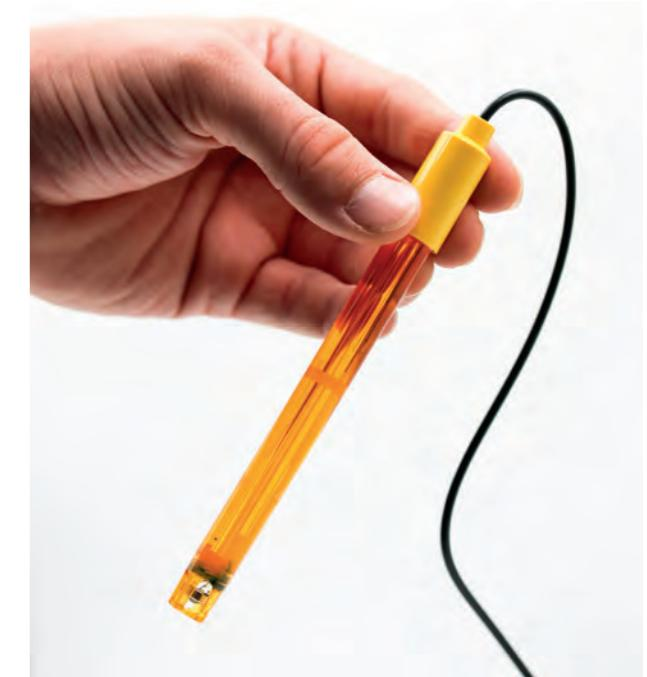
The PrimeLab 2.0 has the option to connect test probes, such as those used for pH, EC, TDS, Salinity, ORP and Temperature. When connecting probes to the PrimeLab 2.0, the photometer manages the probe, obtaining readings which can be stored under the user-defined Accounts (water-sites) and synchronized to the LabCOM®-Cloud (optional).
