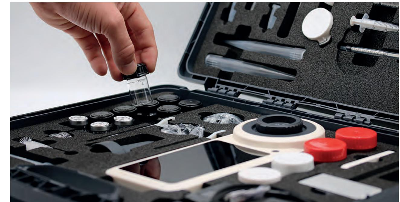
The Water-i.d.<sup>®</sup> PrimeLab 2.0 Pre-Set-Kits offer complete solutions which includes all reagents and accessories for testing the water according to a special application. Combining the accuracy of the PrimeLab 2.0 photometer with suitable reagents enable the user to be fully equipped for
