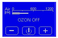
The upper bar graph indicates the volume of the air flow through the device (in I/h).
